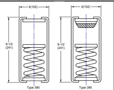
Note: 1. Clearance for a 5/8 dia. rod is standard, for a 3/4 dia. rod is optional.
